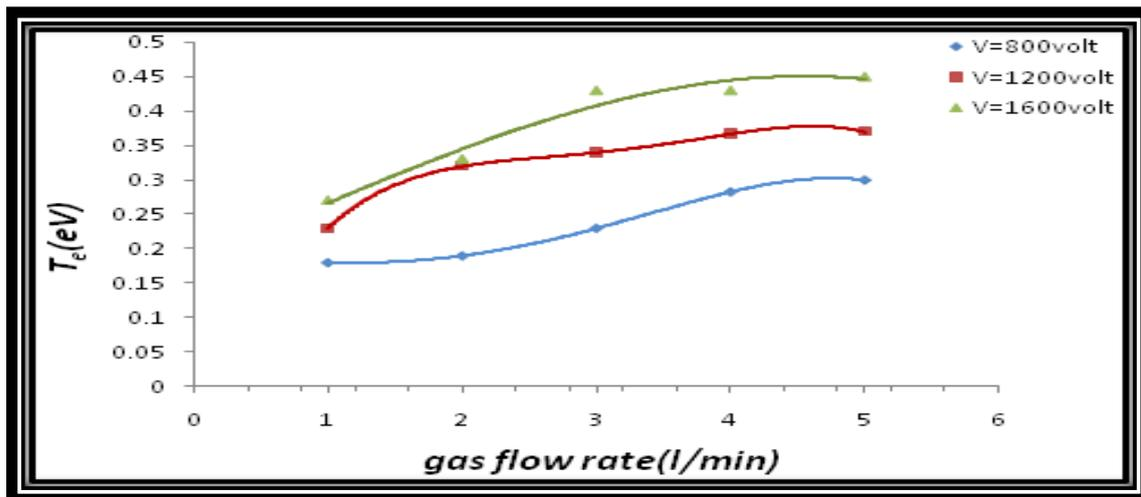
Fig.(3): the relationship between the electron temperature as a function of gas flow rate.
