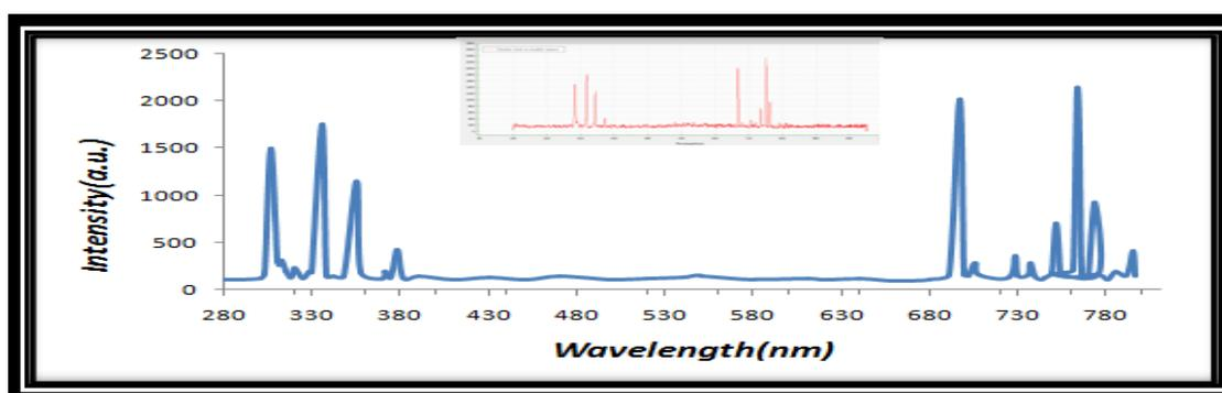
Fig.(2): Spectra of argon plasma jet operated in open air.
