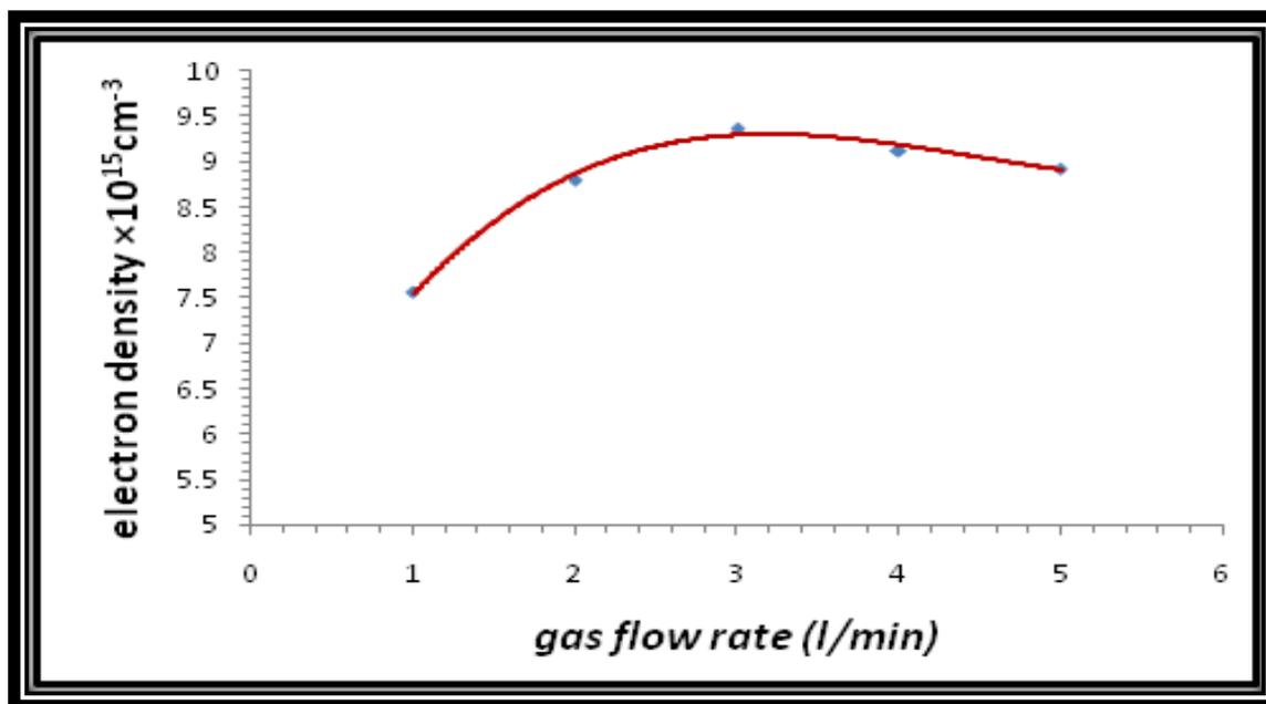
Fig. (4): the relationship between the electron density as a function of gas flow rate.
